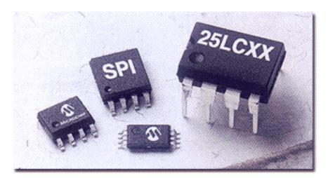
The EEPROM device is a 25LC160A from Microchip. It is a 16Kbit SPI device with a voltage range from 2.5V-5V and is in a 8 pin DIP package. It is organized as 2K x 8bit and has 16 byte pages. There is an active low write protect line that is pulled high. Also, there is an active low hold pin that is also pulled high. The remaining pins are the SPI interface pins which are routed to the HCS12 pins via the Custom Interface Board.
