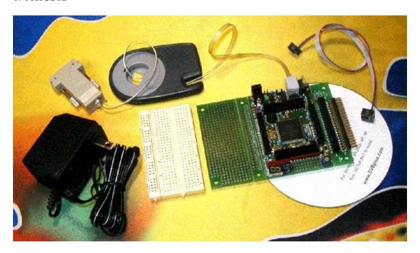
Above is a picture of the MiniDragon+ Development board from www.evbplus.com. This is the board that is used for the Lotus project and it contains a MC9S12DP256. This controller has 256KB of Flash, 12KB of SRAM, 4KB of EEPROM and is internally clocked at 24MHz.
