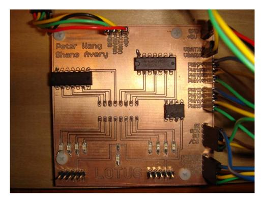
Above is a picture of the Custom Interface Board. The schematic capture and board layout was done in Eagle. The boards were cut using a Protomat machine that plots the layout to X,Y coordinates and literally drills out the non-copper portions of the PCB. It is a two sided PCB in which the bottom (not shown) contains the bypass capacitors and the DIP resistor pack.
